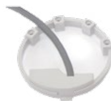
6561RS Pulse emitter REED SWITCH type. 1/10 pulse/liter.
