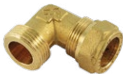
1104FD Bend fitting, nut and olive for copper pipe, male connecting thread with flat seat for corrugated steel pipe and flat washer
