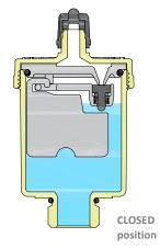
Eliminating the air in the circuits avoids problems such as noise in the system and wear of its components, to ensure better performance of the radiant terminals, resulting in a consequent reduction in operating costs (to learn more, see the "INFORMATION FROM TIEMME" section of this technical data sheet).
